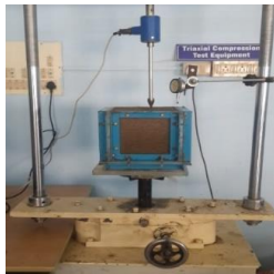
Figure.3. Test Setup of Cone Penetration on sand
